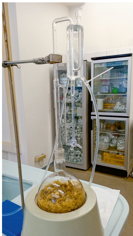
Fig. 1. Hydrodistillation on hop cones in the Deryng apparatus
